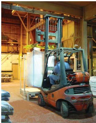
Bulk bag being loaded into top section at floor level
