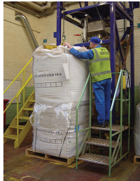
Rigging bulk bag on to lifting frame
