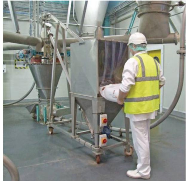
Cocoa powder being dumped into sack tip station
