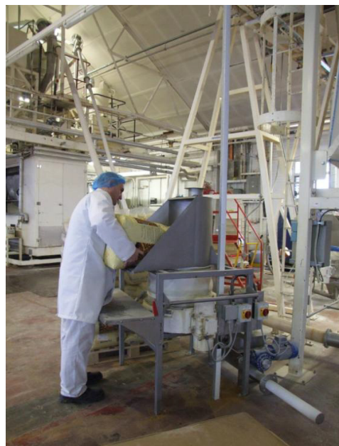
Operative charging sacks of brown flour directly into the mixer via the additional conveyor
