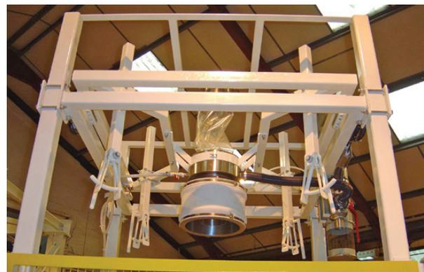
The inflatable filling head and quick release bag support latches are all part of the load cell mounted bag weighing frame
