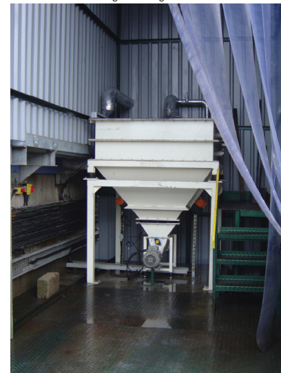
Spiroflow Bulk Bag Discharger inside it's weatherproof housing. Note: The plastic strip curtain is held aside for photographic purposes.
