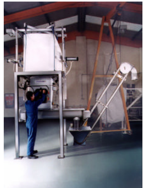
Aero Mechanical Conveyor can be installed vertically or at any angle to suit layout requirements
