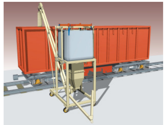
Loading railcars from bulk bags using an aero mechanical conveyor. AMCs can convey at rates of up to 60 tph.
