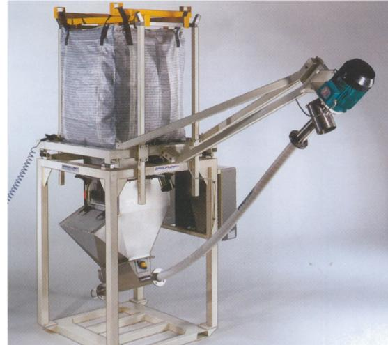
Bulk Bag Discharging System with Static Grounding Device
