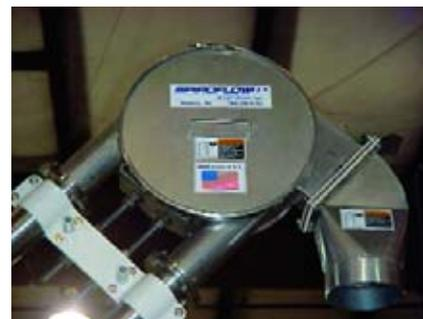
*The resin discharges from the aeromechanical conveyor into a mixing vessel at an even and controlled rate.*
