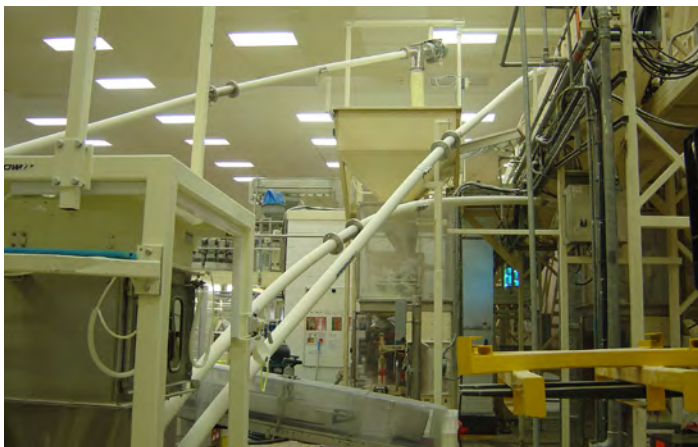
A typical Flexible Screw Conveyor installation.
