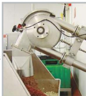
Interlocked inspection hatch in sprocket housing.
