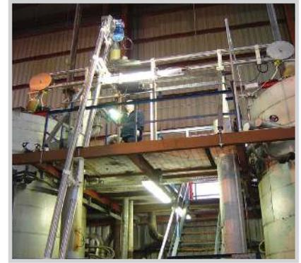
Inclined & horizontal AMCs feed additives to either of two (2) tanks.
