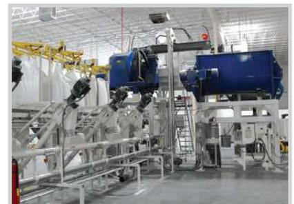
An AMC is used to unload sacks of sugar into a storage hopper.
