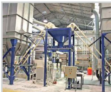
Two (2) AMCs deliver tin oxide from process to packaging.
