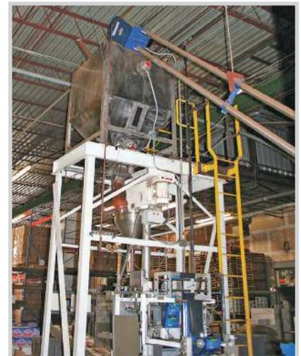
An AMC transfers flavored coffee powder from a blender up to a packing machine.
