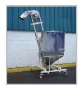
An AMC with a bag dump hopper & integral dust hood.
