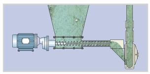
When space is tight, a screw conveyor can be used to deliver material to the inlet chute of an aero mechanical conveyor.
