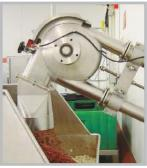
Interlocked inspection hatch in sprocket housing.
