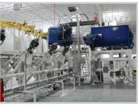
An AMC with multiple inlets delivers cement, sand, ash & recycled glass to a second unit that lifts them up into a mixer.
