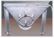
Inlet chute with aeration device
