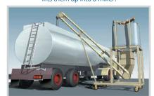
A bulk bag discharger & an AMC load a road tanker truck.
