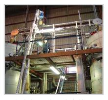
Inclined & horizontal AMCs feed additives to either of two (2) tanks.
