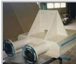
Conveying product through an idler box is not recommended, although idler turns are often used as a product discharge point in a system.
