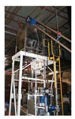
The Aero Mechanical Conveyor delivers coffee blends to the buffer hopper on top of the packaging machine.
