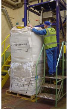
Rigging the bulk bag onto the frame
