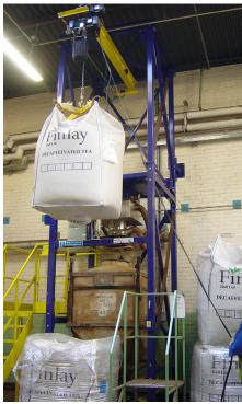
Hoisting the bulk bag into the T6 Unloader
