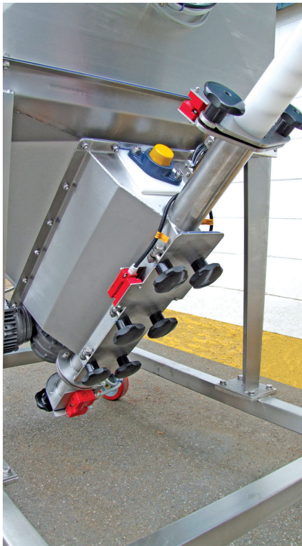
Inlet section of the Flexible Screw Conveyor showing the interlocked, easy to remove access panel for cleaning.
