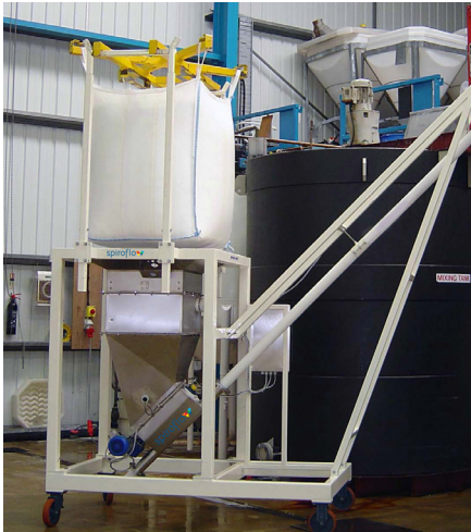
Mobile Flexible Screw Conveyor conveys sugar for liquid blends
