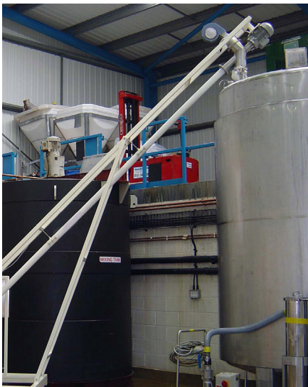
Low pressure blower mounted at the Flexible Screw Conveyor prevents sugar buildup from vapors
