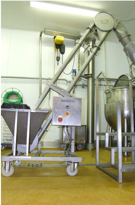
The mobile Aero Mechanical Conveyor transfers Gelatin
