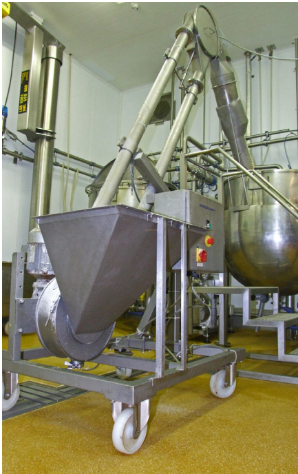
The mobile Aero Mechanical Conveyor transfers Gelatin
