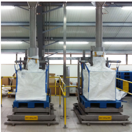
The bulk bag fillers in the 'fall' position
