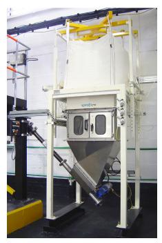
Bulk Bag Unloader with a Flexible Screw Conveyor leading off to the left
