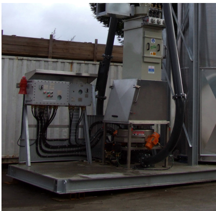
A safe system for unloading, conveying and storing Hydrated Lime (Calcium Hydroxide)
