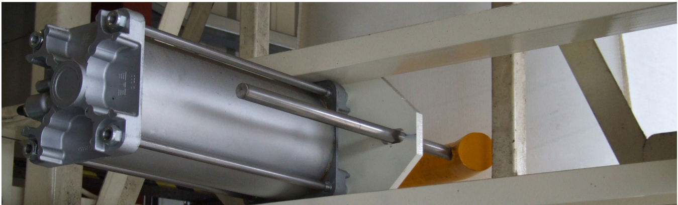
Heavy-duty Bulk Bag Massagers installed on the Side of the Bulk Bags
