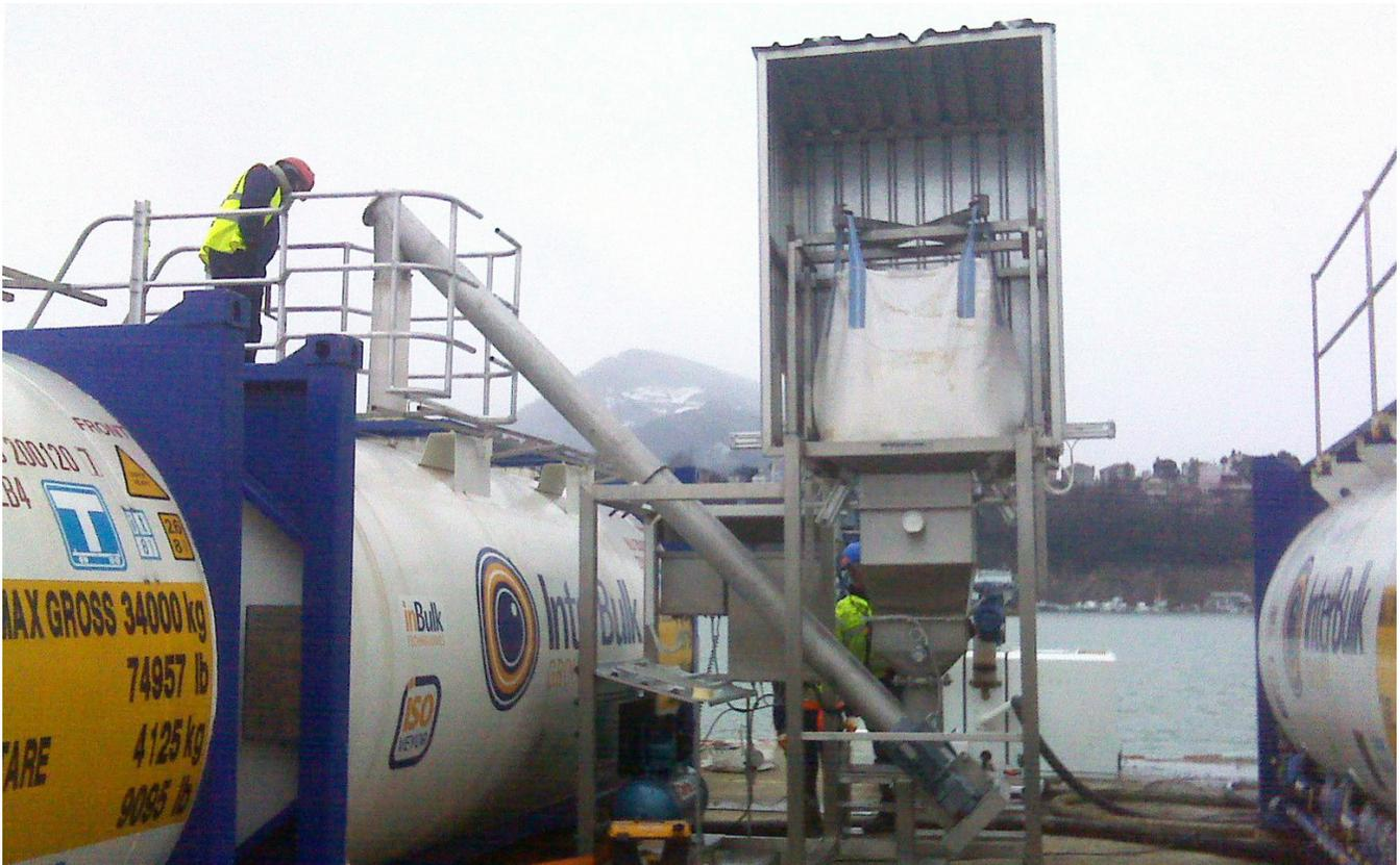
Dockside ISO Tankers are filled with a Spiroflow Bulk Bag Unloader.
