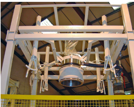
The inflatable filling head and quick release bag support latches are all part of the load cell mounted bag weighing frame.
