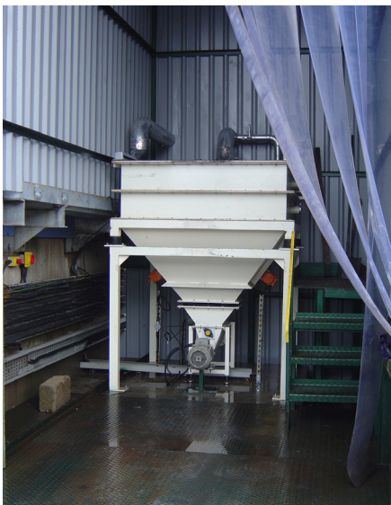
Spiroflow Bulk Bag Unloader inside it's weatherproof housing. Note: The plastic strip curtain is held aside for photographic purposes.
