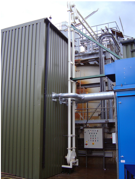
Spiroflow Aero Mechanical Conveyor transfers product from the Bulk Bag Unloader to a very large mixing Tank
