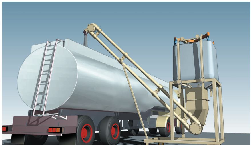
Product can be fed into an aero mechanical conveyor from a bulk bag (as shown above), silo, blowing line or mechanical shovel.
