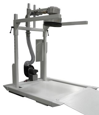
Bulk bags can be easily be filled with Spiroflow's 'Low Loading' Bulk Bag Filler. A special low loading ramp and low profile pallet base makes unloading filled bulk bags a simple operation with a pallet truck.
