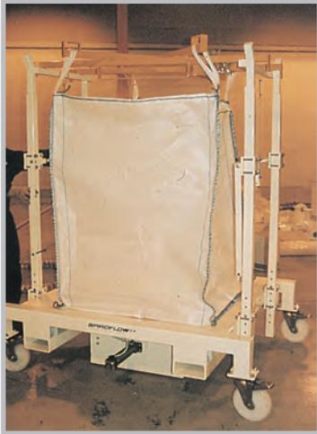
This useful device, often used with a Type 5 Low Loader, can also be supplied as a storage frame for bulk bags. If located on a mezzanine, it can provide direct loading into packaging or process machine hoppers.
