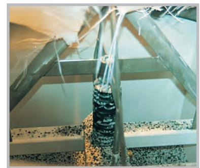
3. The bag is ruptured by the knife and product flows from the discharge dish into the integral transfer conveyor.
