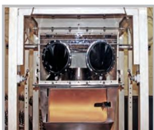
A glove box arrangement for untying bags containing hazardous product, preventing operator exposure to product.
