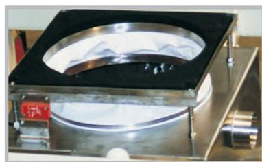
The discharger base unit has a dust-tight docking seal on to which the top frame and bulk bag is placed. A spout clamp allows the bag to be untied without dust emission or spillage via an access door.
