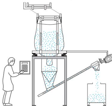
Our specialized batch controller provides both 'bulk' & 'trickle' feed for loss-in-weight dispensing. The Pause-Resume feature pauses the discharging operation when one bulk bag is empty and retains in memory the amount dispensed. When a fresh bulk bag is placed on the discharger, the controller recalls the remaining weight required and resumes discharging.
