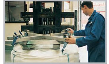
2. The bag is lifted by a forklift truck on to the robust bulk bag support frame. Spring-loaded arms on the bulk bag support frame gradually raise and tension the bag during emptying. This ensures total emptying of the bag and prevents the bag spout or liner from sagging or fouling the take-off conveyor.
