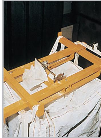
Bulk bags are often supplied with long inner liners which require clamping at the top to prevent fouling the take-off conveyor.
