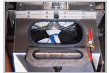
4. The pneumatically operated massage system, adjustable in position for optimum effectiveness, ensures consistent flow of difficult products.
