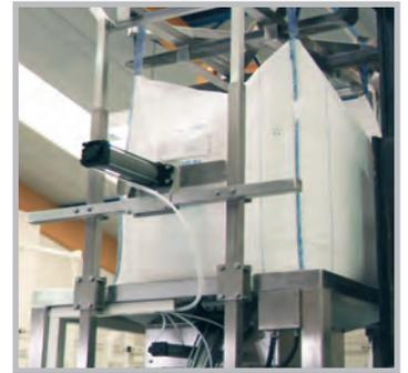
3. The integral chute has an access door for easy bag untying. The spout closure bars ensure the bag remains tightly closed until the emptying process starts.
