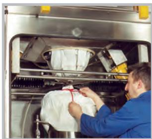
Spout closure bars have several functions: they prevent dust by allowing untying of the bag without product release; their aperture can be set to control the flow rate from the bag; they can close off the spout if used in a batch weighing operation; they allow the bag to be re-tied and removed from the discharging frame.
