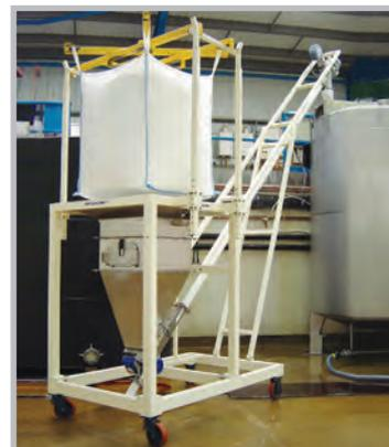
A robust mobile frame, with towing facility if required, provides a versatile arrangement for processors who require discharge of bulk bags at several locations. (This option is not available for Type 6 with Integral Hoist).
