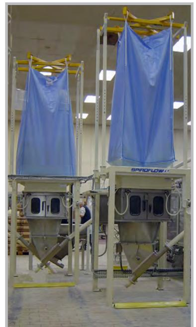
Good Health & Safety practice requires, as a minimum, that the weight of a bulk bag be supported as it is unacceptable to support bags from their loops for any length of time where operators are present. It is certainly not good practice to use a forklift truck to hold a bag over a point of discharge. Additionally, it ties up the forklift preventing it from being used elsewhere.
