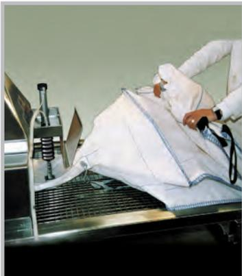
A bag folding table provides a practical solution to bag disposal problems and allows extraction of residual product from the bulk bag.
