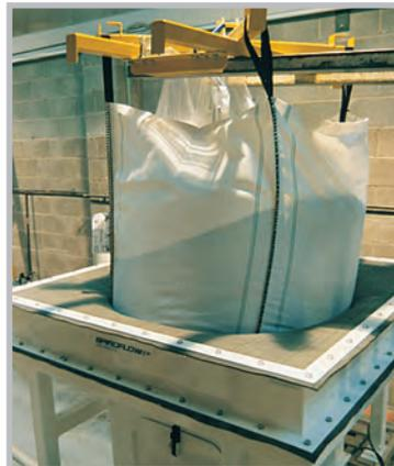
2. The double membrane ensures that the bag sits deep within the dish and no dust escapes during discharge.
