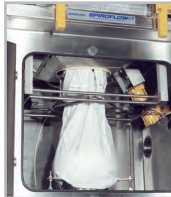
The pneumatic stretching and sealing device assists the flow of poor flowing or very light product through the bag spout and into a downstream vessel, valve or conveyor. It also provides total dust containment of dusty or noxious products.
