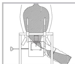
Liners can be removed from the bag after discharge and contained without emission of dust with use of this powered retraction device and compaction facility.
