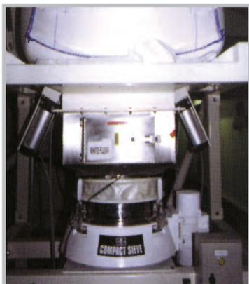
An integral vibratory sieve provides assurance that product from a bulk bag is suitably screened for lumps and other impurities before entering the discharge chute.
