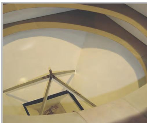
1. The T4 consists of a robust frame and discharge dish with a knife to pierce the base of the bag. A double membrane with dust extraction facility ensures total containment of dust emitted during the bag piercing operation.
