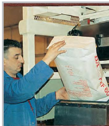
We can supply a large bag/sack tip door so that if your supply of bulk bags is interrupted, delivery of raw materials can be accepted in small bags/sacks and handled by the Spiroflow discharger.
