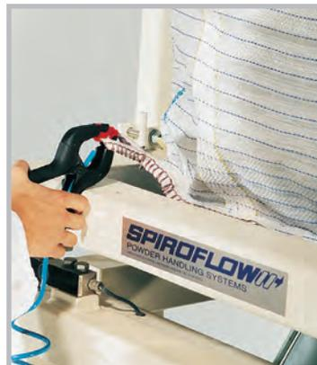
Designed for use in hazardous atmospheres with a Type C static dissipative bag, the earth monitoring device automatically checks that the bag is correctly earthed before discharge can commence.
