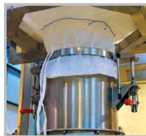
Our Hygienic Liner Clamps offer easy management of loose liners preventing product spillage and, combined with the tensioning action of the spring-loaded bag support arms, prevent the distension of the liner into downstream equipment. When housed in a cabinet under negative pressure, they offer 'total containment'.
